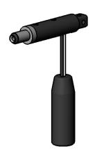
MA039201 is a highly durable test plug for testing 2.0-2.1/5.5mm DC-connector interface. It has a DC-jack with 2x0.50mm<sup>2</sup> cable for easy integration. Length of the cable is 300mm.
