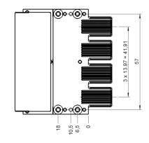
MA092617 8P8C x4 Modular Test Connector is a straight signaling test plug for 4-port RJ45 interface testing. Suitable for all devices with 13.97mm pitch 4-port RJ45 connectors, like Ethernet routers, Ethernet switches and others.
