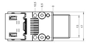
BLUELEC HDMI Test Connector MA089770 is a 19-pin test connector designed for testing of HDMI Type-A interface. The transmission of high data rates can be achieved, recommended to be verified by our customers in their applied test setup.
