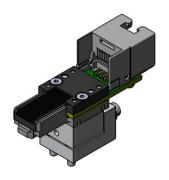
When using float with Test Connector MA014781 the mounting screws need to be installed from opposite side of default configuration. It is recommended to change the default countersunk screws to M2x12 mm cap head screws. Also dowel pins need to be pressed to opposite side.
