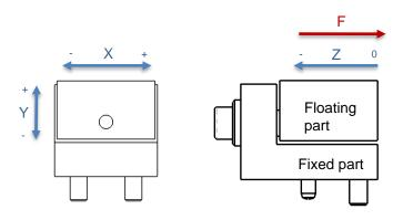
Default position of floating part is '0' for all axes. Displacement of Z is needed to allow displacement of X and Y.
