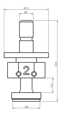
MA040494 is a capacitive test finger designed for various touch screen testing, with durable rubber tip.
