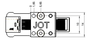
MA024613 USB Type-C Test Connector is 24-pin double sided connector with straight signaling. It has 0.75mm longer tip than our standard USB C Test Connector to achieve proper connection to DUTs with thicker casing.
