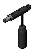
MA009073 is a highly durable test plug for testing 2.5/5.5mm DC-connector interface. It has a DC-jack with 2x0.50mm<sup>2</sup> cable for easy integration. Length of the cable is 300mm.
